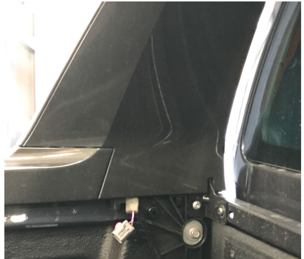
Fig2. 2018 Model onwards. Has no access panels in the front corners.
