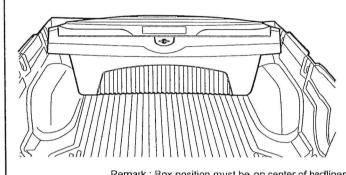
Remark: Box position must be on center of bedliner.
