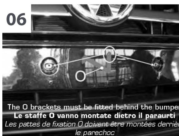
The O brackets must be fitted behind the bumper
