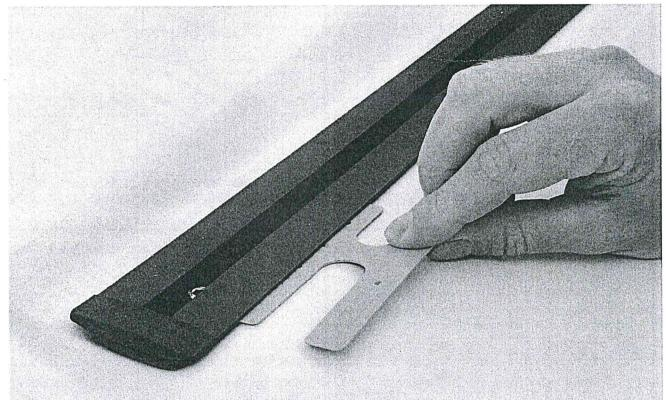
Use gauge supplied to check clearence from channel to lid. Gauge should fit easily.
