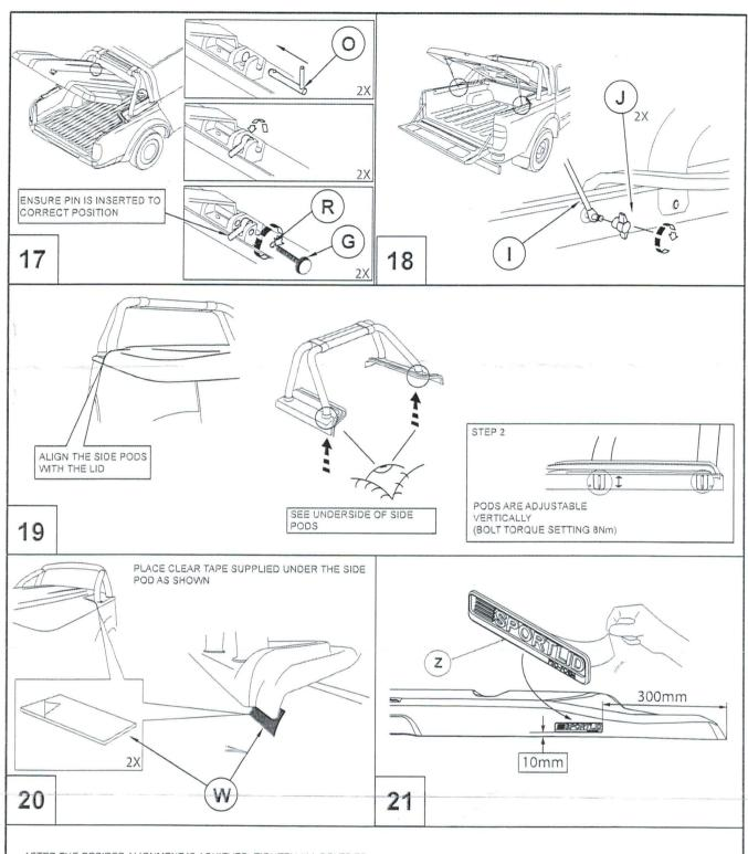
AFTER THE DESIRED ALIGNMENT IS ACHIEVED, TIGHTEN ALL BOLTS TO THE REQUIRED TORQUE SETTINGS AS STATED IN THE INSTRUCTIONS
