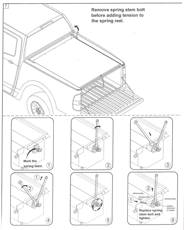
Fully rotate spring stem (see mark) - 14 times
