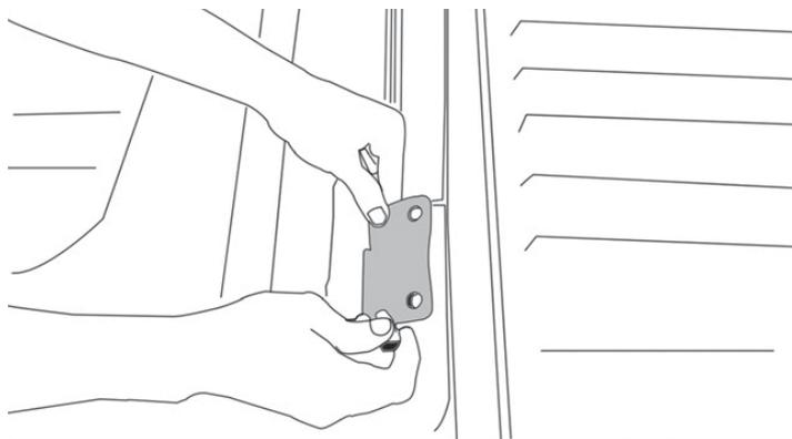
02. Put ProLift brackets with the tailgate using original bolts.
