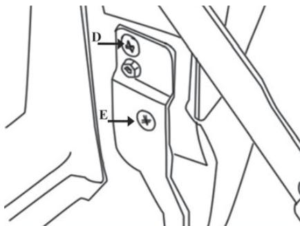
07. Attach damper bracket to the tailgate using original bolts.
